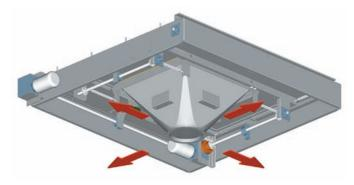
Dual direction positioners are used to move standard duty loading spouts horizontally in the X and Y axis when loading trucks or railcars. Dual direction positioners allow the driver to stop the vehicle in the designated loading area without having to be precise. The loading spout can then be positioned directly above
