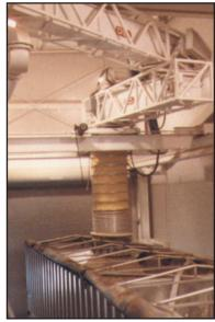
DCL offers a large selection of articulating positioning arms that provide horizontal travels up to 60 feet [18.3 m] by 6 feet [1.8 m]. Conveying arms can be provided as aeration conveyor, en masse, and screw conveyor configurations.
