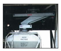
positioners allow the driver to stop the vehicle in the designated loading area without having to be precise. The loading spout can then be positioned directly abovet he vehicle hatch. DCL offers a selection of rotary positioners that provide radial horizontal travels from 4 feet [1.2 m] in diameter up to 12 feet [3.6 m] in diameter.
